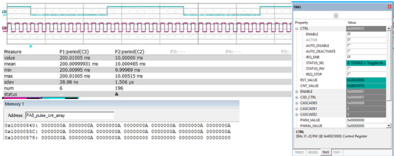
Figure 14 - Scope capture with MCU RAM and register information for input pulse count. A) Waveform showing the interval for counting pulses and the actual pulse train. (Note 10 pulses per half period of the window), B) Memory display window from debugger showing the 16 entry array with pulse count and C) TIM3 register contents to count pulses on PA[8]
