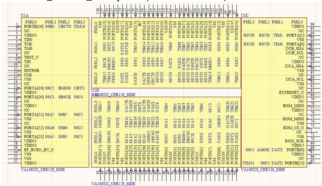
Figure 9 VA108XX_CER128_Side symbol (Alternate 1 mode)
